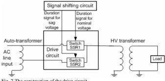
Fig. 7 The construction of the drive circuit
