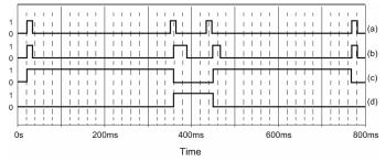
(a) Four special pulses provided to the signal shifting circuit from the duration control circuit
