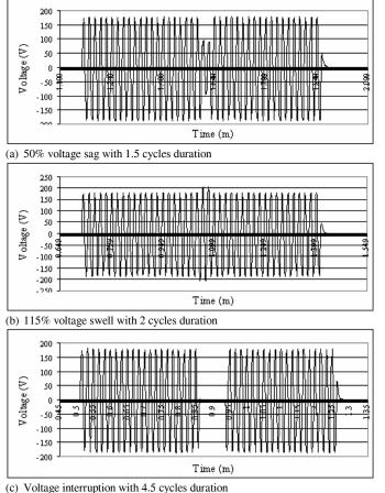
Fig.8. VSG operation results captured by digital scope
