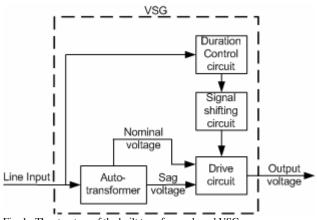
Fig. 1. The structure of the built transformer-based VSG
