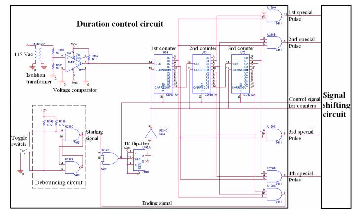
clock signal for the second counter. The carryout output of the second counter (100 cycles duration and 0.5 duty ratio) acts as the clock signal for the third counter.
